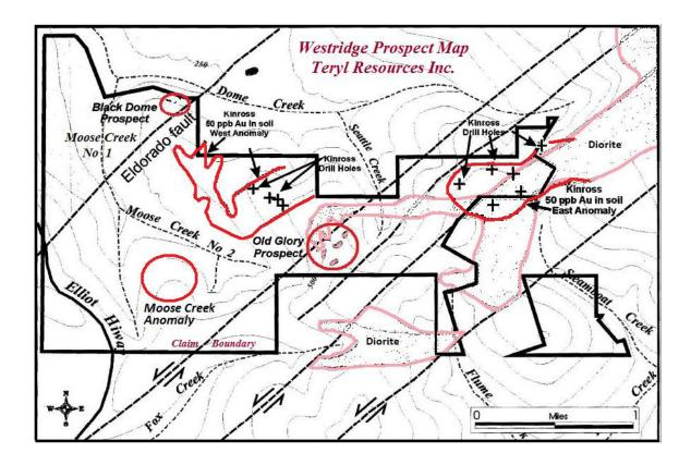
Mineral exploration consisted of up to 610 metres (2,000 feet) of shallow core drilling utilizing a narrow diameter AQ core drill to initially test lode targets on the Old Glory Prospect and Moose Creek Anomaly. On positive results, a larger scale reverse circulation drill program will be conducted.
